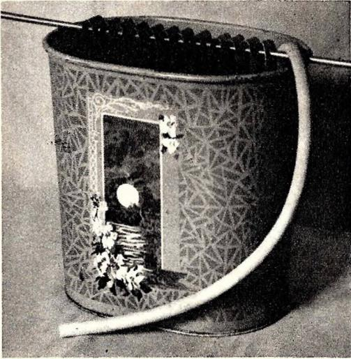
**AN EFFICIENT WASHING TANK.** A tin waste basket can be converted into a practical washing tank for film-pack or cut film. Be sure to seal any leaks in the edge before attempting to use it.
