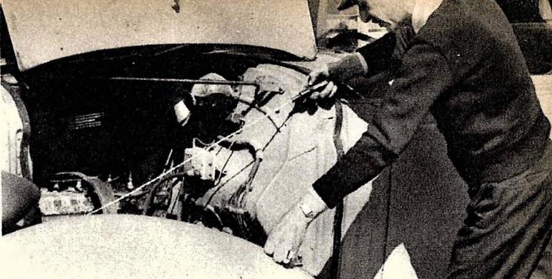
When bolts, nuts or other metal parts have to be removed from narrow or inaccessible places, this narrow garage-type magnet will be very useful.
