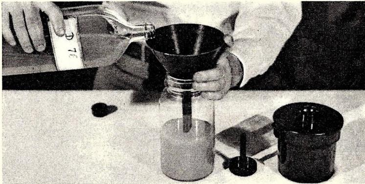
No. 2: Filter amount of developer required by tank, using wad of cotton in large funnel. Old fruit jar better than bottle; supports funnel more securely. Adjust developer temperature by immersing jar in hot or cold water. Most formulas call for 65 degrees F.
