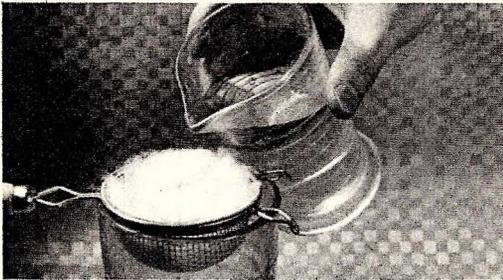
**FILTERING DEVELOPER QUICKLY.** When time must be saved, solutions can be filtered quickly by using a nickel-wire strainer lined with a layer of cotton. If the strainer is not nickel plated, it should be coated thinly with asphalt varnish.
