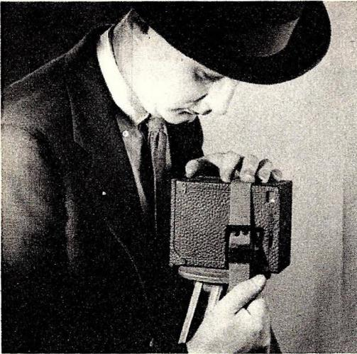
**ATTACHING BOX CAMERA TO TRIPOD.** When the lens aperture of a box camera is stopped down, and time exposures used, the results frequently are as good as can be obtained with a more expensive camera. The camera can be mounted securely to the tripod with a luggage or book strap.
