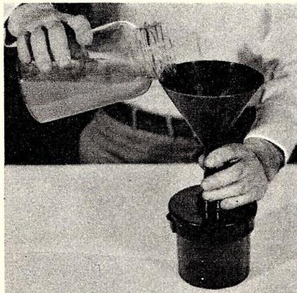
No. 3: Rinse funnel well. Note time, then pour in developer slowly, giving air plenty of time to escape. Rinse funnel and jar thoroughly, invert on sink to drain.
