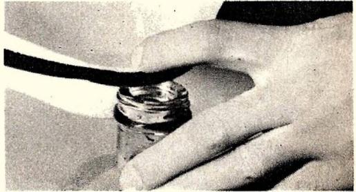
**MOISTENED LIP OF TRAY AIDS POURING.** When pouring from a pan or tray into a bottle, it is difficult at times to start the flow in the right direction. If the lip of the vessel is moistened, the fluid will follow the trail of moisture and not spill out at an unexpected point.
