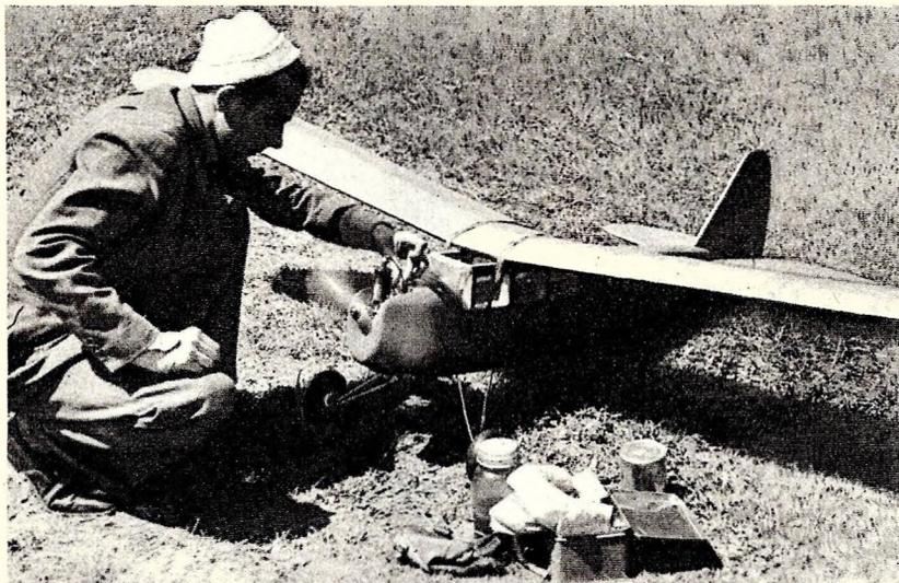
Left—Many a contest is won in the "pits", the roped off areas where the modelers are permitted to adjust the miniature gasoline engines of their entries. The adjustment of the carburetor needle-valve often means success or failure of the flights.
